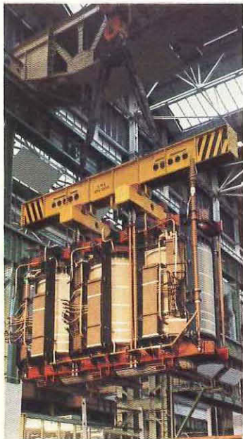
The completed core and winding assembly of an 250 MVA auto-transformer being lifted for fitting into its tank at GEC Power Transformers Ltd Stafford.
