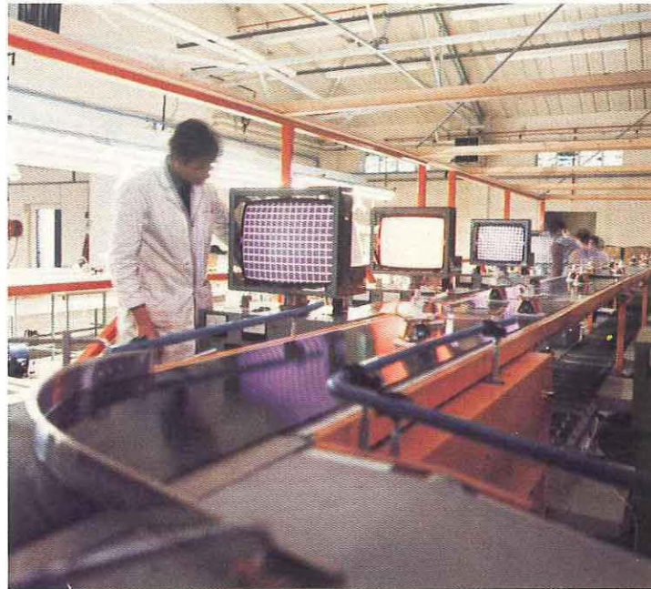
Deflection yokes being adjusted at GEC-Hitachi Television Ltd. The television sets seen in the picture are part of the test equipment.
