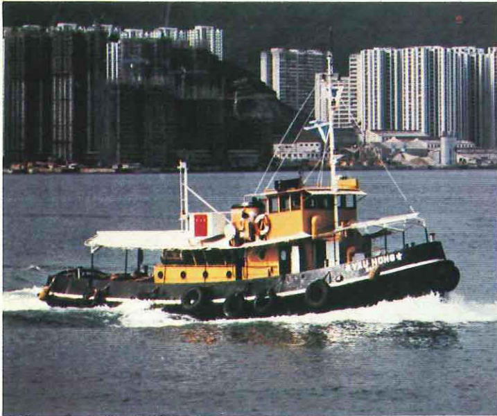
A tug operating in Hong Kong harbour and powered by a diesel engine made by Kelvin Diesels Ltd Glasgow. The engine develops 440 bhp at 1200 rev/min.
