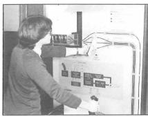
One of the many areas of research is optical data transmission. This is an advanced 'fly-by-light' test rig
