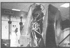
One of CQD's activities - Testing an AEW Radar Scanner on the 134 KN thrust vibration system
