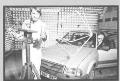
Setting up a vehicle for EMC testing to demonstrate its ability to withstand high RF
