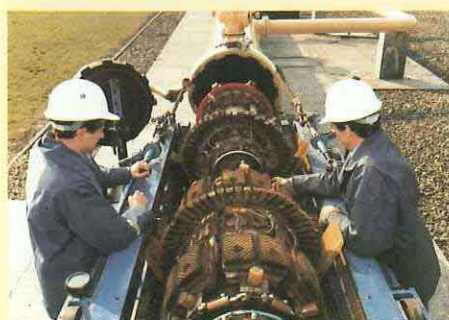
The "Intelligent Pig" for British Gas incorporates magnetic tape data recording equipment for remote inspection of pipelines.
