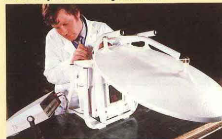
This J-band radar is used underground to detect the level of coal in storage bunkers.
