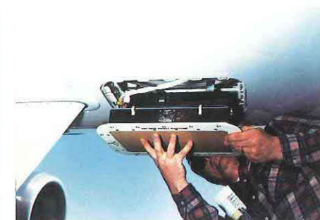
AD 660 Doppler Velocity Sensor, an effective groundspeed measurement system for airliners, can also be used in tactical navigation.
