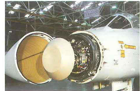
Foxhunter AI radar is an advanced multi target track-while-scan system in service on Royal Air Force Tornado fighters.
