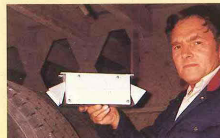
Doppler Velocity Sensor for road vehicles measures groundspeed by radio beams as in aircraft dopplers. Sensors have been supplied for magnetically-suspended train systems.
