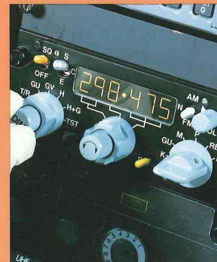
The AD3400 multimode communications system, adopted by British and overseas air forces, can cover all VHF/UHF bands, AM and FM.
