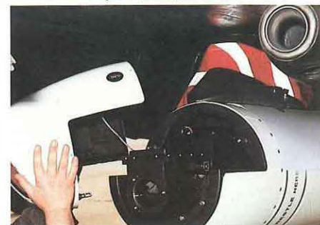
High-performance FLIR pods, based on interoperable TICM II modules, equip subsonic and supersonic aircraft and are chosen for RAF Harriers and Tornados and the USMC AV-8B.
