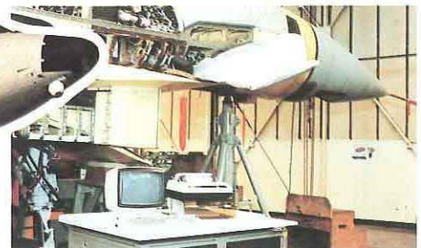
MIL STD 1553B systems integration and test facility in use on the UK's Experimental Aircraft Programme (EAP).
