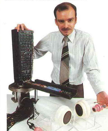
Getting oil ashore from satellite wells in the BP Magnus field depends on these "fail safe" controls and high integrity data links from each wellhead to the platform. This technology derives directly from military aircraft control systems.
