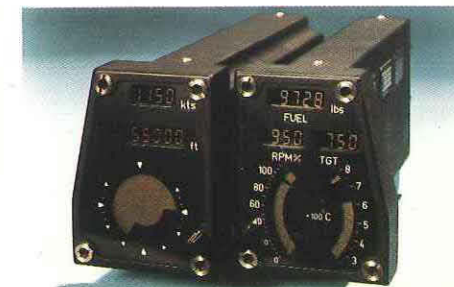
Reversionary instruments for aircraft are a unique application of liquid crystal displays.
