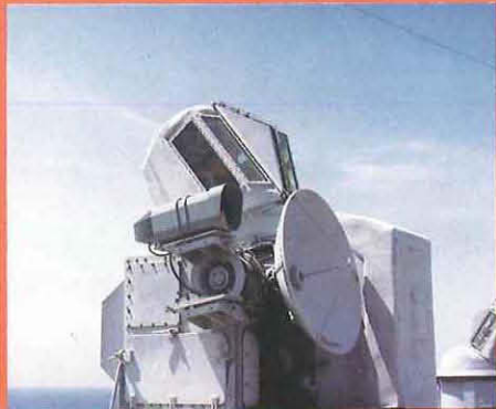
Specialists in thermal imaging systems, we supply this V3800 shipborne imager to several nations. It is one of the many applications of Thermal Imaging Common Modules.
