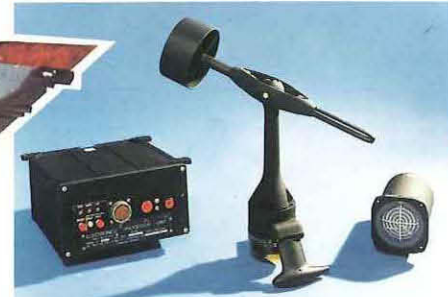
This unique Helicopter Air Data System measure airspeed and direction accurately, right down to the hover, on Bell Helicopter Textron AH-1S aircraft of the United States Army.
