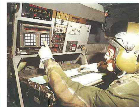
AQS902 Lightweight Acoustic Processing and Display System, LAPADS, is in service on Royal Navy Sea King Mk 5 helicopters. This system can operate with free sonobuoys, or dipping sonar.
