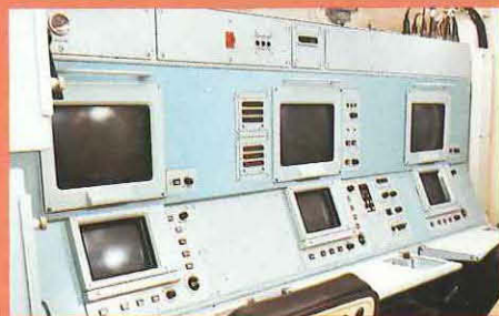
Shipborne processing and display systems for ship and submarine sonars, in service with the Royal Navy and other navies, are microprocessor based and the display consoles have touch operated displays and controls.
