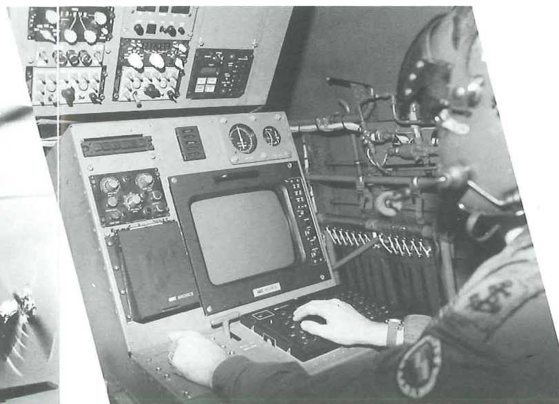
The latest GAv acoustic processor, which equips the Royal Navy Sea King Mk6, entered service earlier this year.
