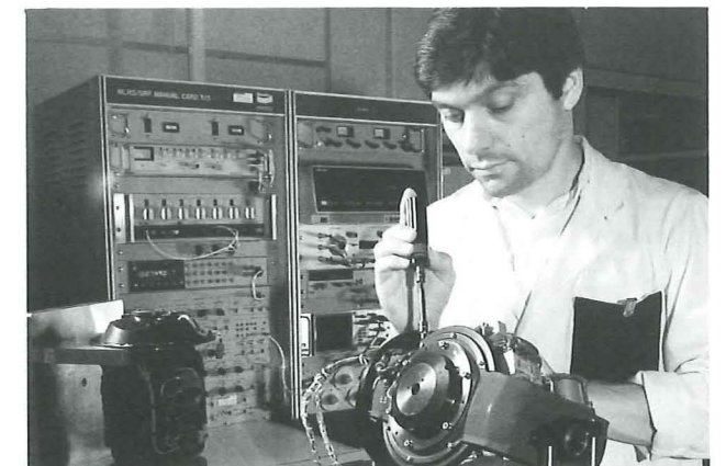
Assembling the gyroscopic elements for the inertial platform of the MLRS.
