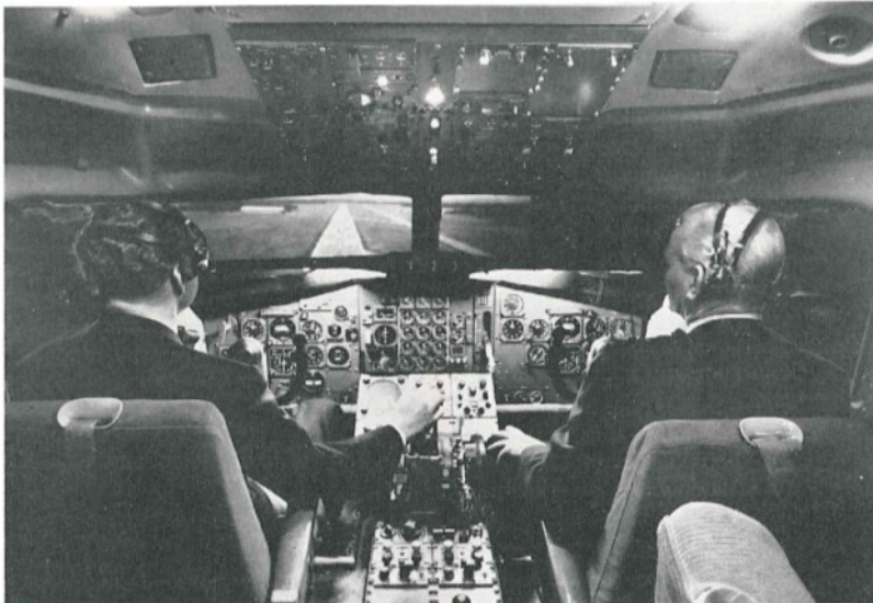
The flight deck of a Trans World Airlines flight simulator showing the visual flight attachment presentation
